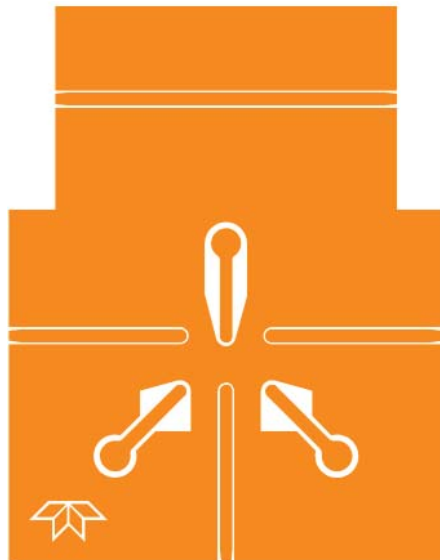
Circuit Side Copper Pattern
